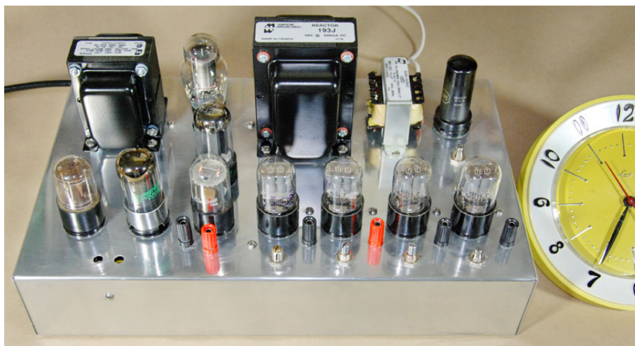
Figure 28 Vacuum tube replica of an early quartz clock (source: tronola.com)
