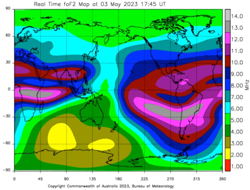
Figure 48 Critical frequency map in the absence of a solar wind storm
