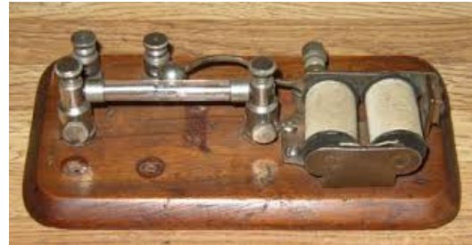
Figure 6 Marconi's 1896 spark gap receiver (source: Wikipedia)
