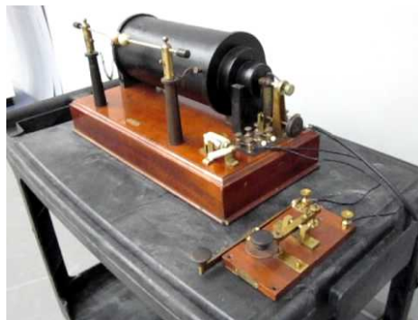
Figure 5 Marconi's first spark gap transmitter (source: author & Wikipedia)
