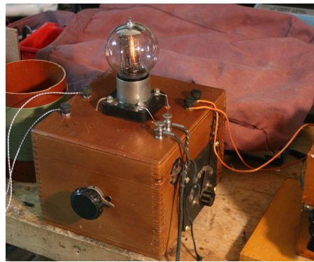
Figure 20 Regenerative receiver (source: Wikipedia)
