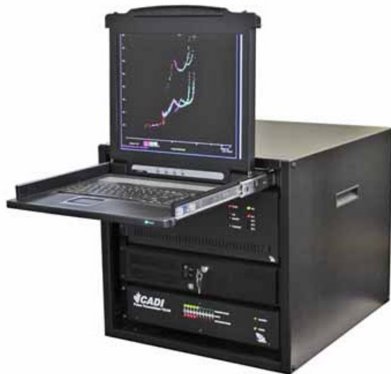
Ionosonde controller & data processor
