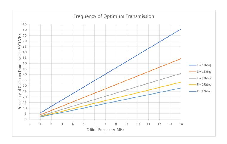
• The following steps are used to determine the Frequency of Optimum Transmission (FOT) to reach a desired destination radio station
