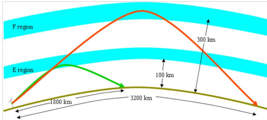
Figure 8 E and F mode propagation (source: Space Weather Service)
