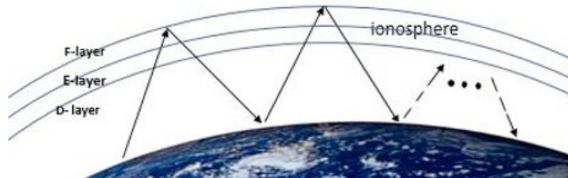
Figure 1 Multiple hop propagation through the ionosphere (source: ResearchGate)
