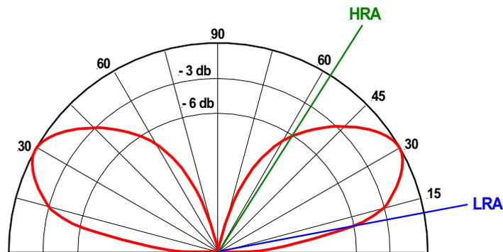
Figure 5 Radiation pattern for a typical 20 meter Inverted-V antenna (source: author)
