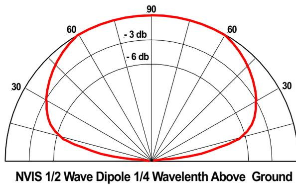
Figure 19 Elevation pattern for an NVIS 40 meter antenna (source: author)
