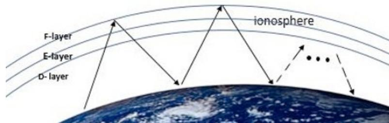
Figure 21 Multiple hop propagation through the ionosphere (source: ResearchGate)
