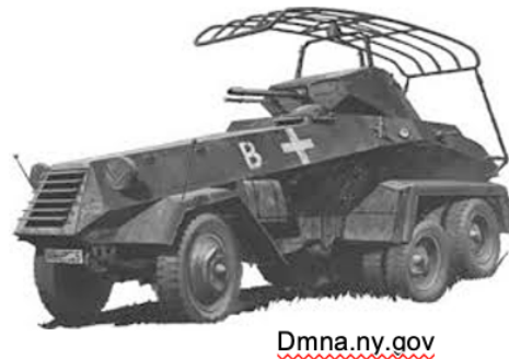
Figure 16 NVIS equipped German armored car
