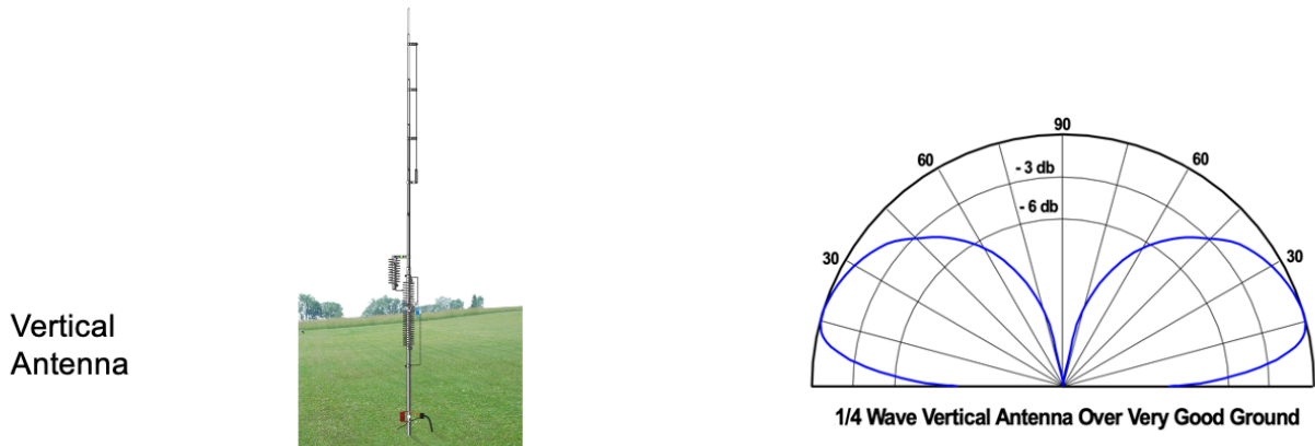
Figure 29 Vertical antenna radiation pattern (source: author)
