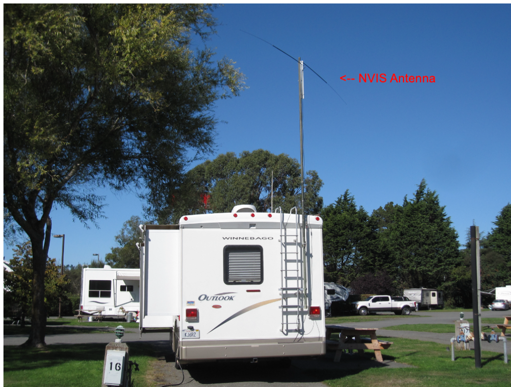
Figure 36 Author's RV configured for NVIS operation
