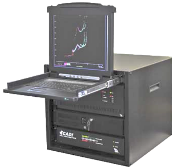
Figure 24 Ionosonde controller and data processor (source: Electronics Notes)
